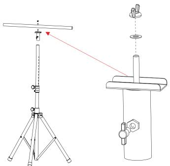
The TOP1 can be mounted onto any 35mm stand. It has been designed to be used in addition with the Novopro BAR1 extension bar but it can used with any suitable extension bar
